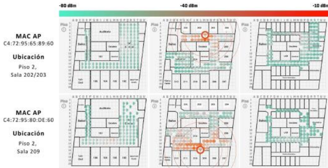
Figure 16 Graphical result of RSSI measurements of 2 selected access points on floor 2 and their effect on floors 1 and 3.
